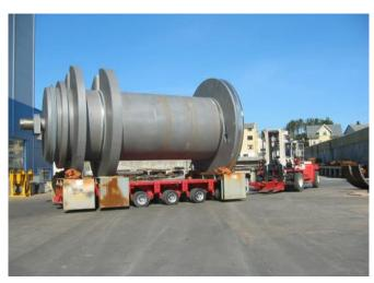
When handling and producing heavy components, the internal transportation logistics are of severe significance. Thus we have invested in several high capacity forklifts and hydraulic carriages.
